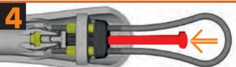
(4b) Absolute safety during fine adjustments. Even when not tightened tightly, the screw itself serves to fully secure the connecting pieces.
